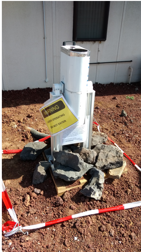
Figure 2.4: Leosphere ALS-450 UV-depolarisation lidar setup during the field campaign. (7.97° S, 14.35° W)
