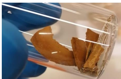
Figure 14. Recrystallized \text{Pd}(\text{NO}_3)_2 with fuming nitric acid agent, dried in vacuum. No bright chunks of Palladium or Palladium nitrate are visible any more.
