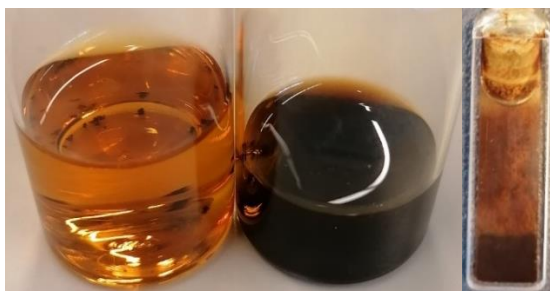
Figure 20: From left to right: 0.1M Pd(NO 3 ) 2 in 1M HNO 3 , 0.1M Pd(NO 3 ) 2 in 0.1M HNO 3 and a 0.1 cm diameter sized UV-vis cuvette filled with 0.1M Pd(NO 3 ) 2 in 0.1M HNO 3 after UV-vis measurements.
