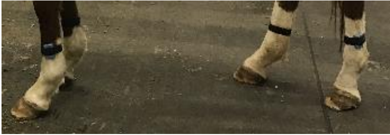
Figure 2. IMU placement on the cannon bones. The Left Front IMU was placed 4 cm proximal to the fetlock joint and the other three were placed on the other limbs at the same height as that Left Front one, measured from the ground.
