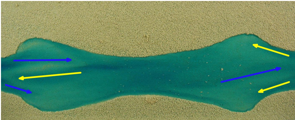
Figure 4.5: Forking channel pairs at both ends of experiment 12.
