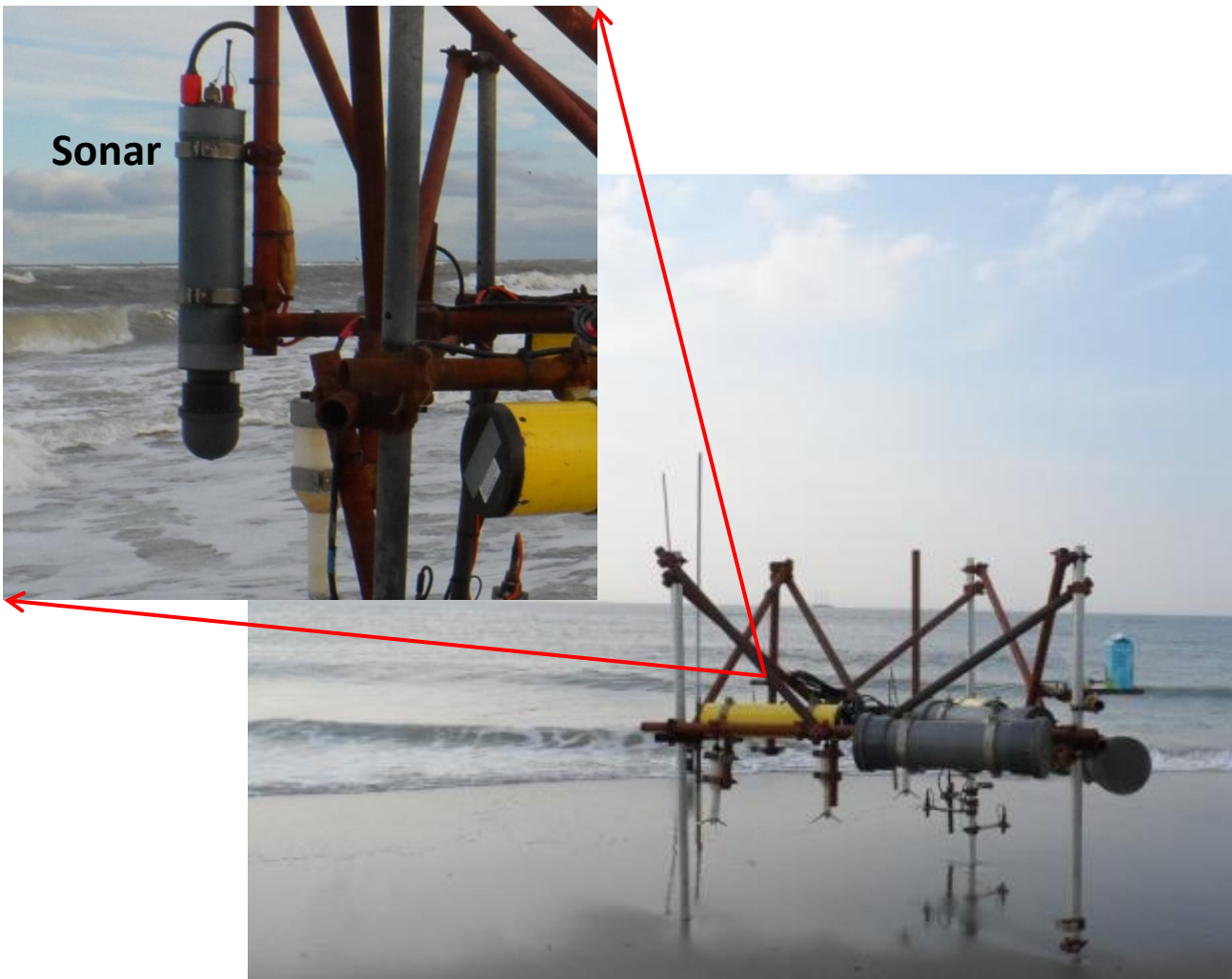
Figure 13. An overview of the rig in the field. The sonar was attached at the seaward side of the frame, like the other instruments. Here the measurements were least disturbed by the frame.
