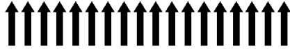
(a) One of the two ground states of the one-dimensional ferromagnetic Ising model
