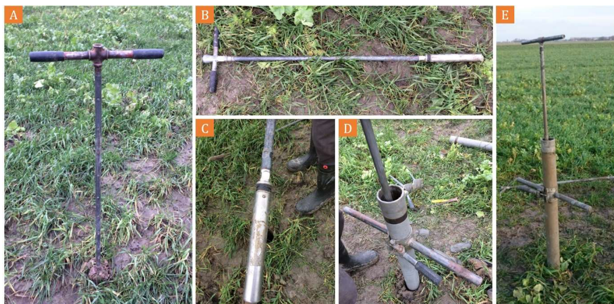
Figure 3.2: Equipment used for the soil sampling. (A): Edelman drill. (B) and (C): Akkerman core sampler and Akkerman tube, respectively. (D) and (E): Equipment used to remove the mud and achieve greater depths.
