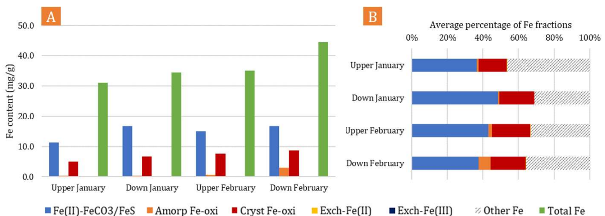
Figure 4.27: Left (A): Fe content in various fractions extracted in all ditch samples. Right (B): Total Fe composition as the average percentage of each fraction extracted from the ditch samples.
