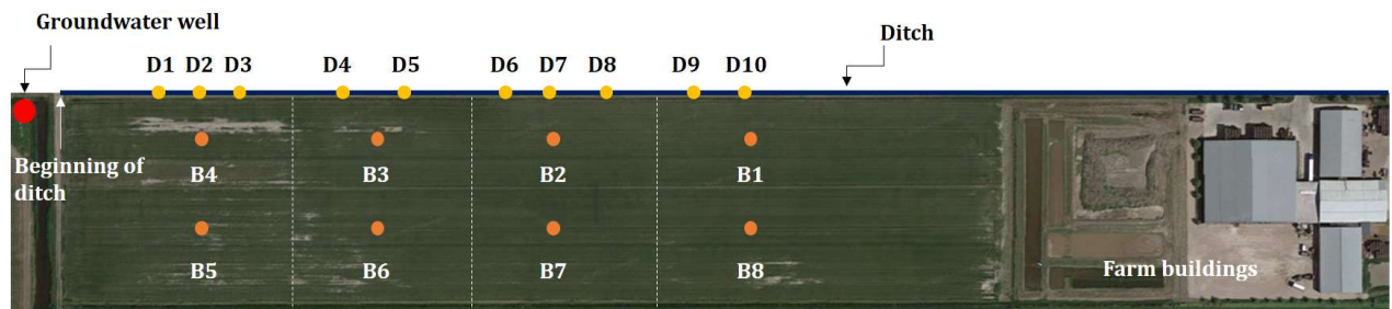
Figure 3.1: Scheme with the arrangement of boreholes (B1-B8) and drains (D1-D10) in the study area. The white dashed lines determine the limit of influence of the boreholes and their respective drains. This arrangement was used to create the mixing lines shown in the results section.
