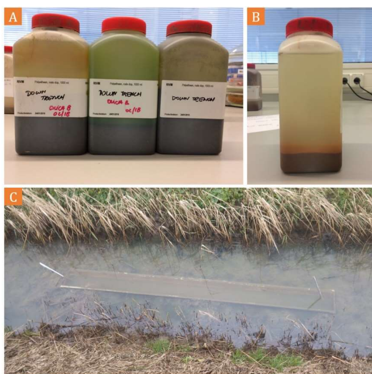
Figure 3.3: (A): Ditch settled material. (B): Drain slurry. (C): Trench used to collect ditch sediments.
