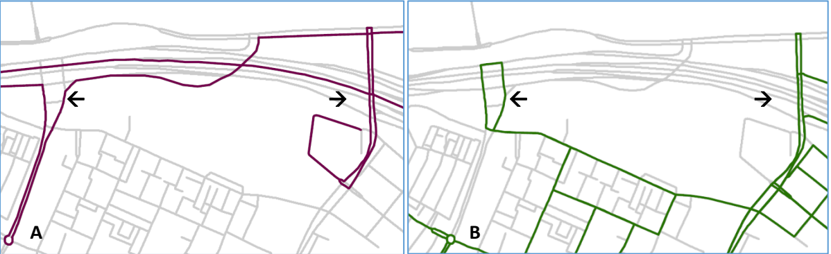
Figure 5.4 zoom in on the A15 motorway exists. (a) Route 1 services both motorway exits, but (b) route 2 also services these arcs. Motorway exits indicated by the black arrows.
