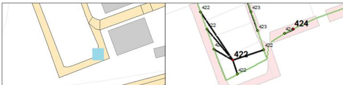
Figure 4.10 Adding critical frost spots (blue polygon) for phase B. Figure 4.11 Manual checking if the centre of the TOP10NL road parts (red points) connect to the centre of the TomTom lines (green points) via the black plotted line.
