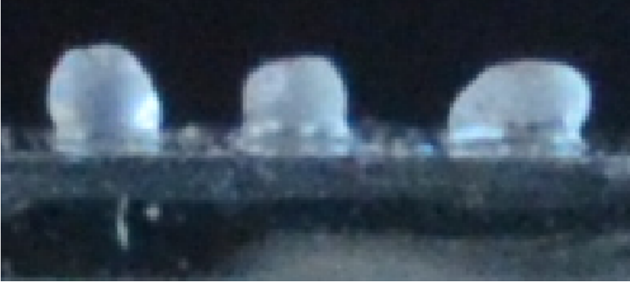
Figure 5: Photograph from the side of a sample, used for calculating the radius of curvature.
