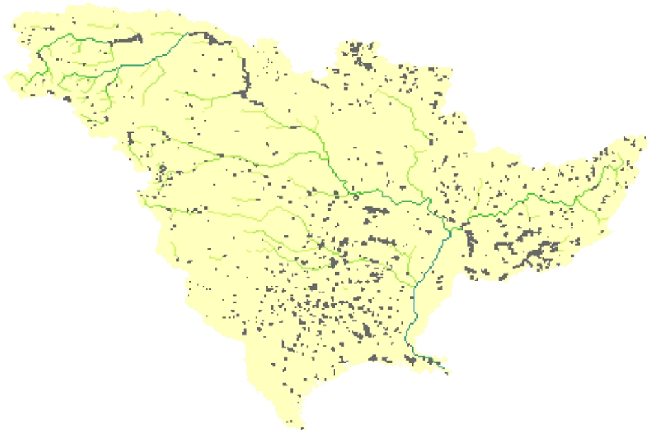
Figure 5.10: Average annual sediment transport for the all catchments in the MRB in [MT/yr].
