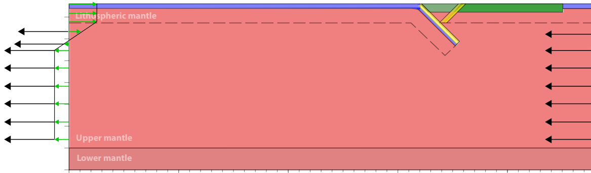
Figure 7: The velocity boundary conditions for each model set up. The overriding plate is kept fixed, while there is a small convergence velocity of the subducting plate (green arrows). There is an equilibrium in inflow and outflow of material. The black arrows indicate the mantle wind.
