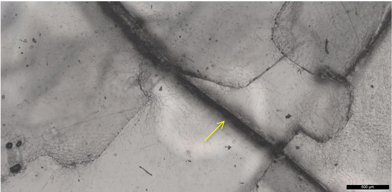
Figure 8: Reflected light, intergranular crack (yellow arrow) and well developed subgrain structure, deformed rock salt (SP205-1).
