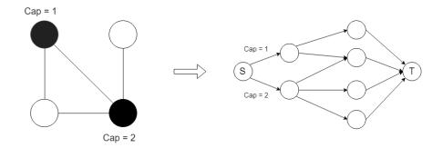
Figure 2: A bipartite flow graph. On the left the original graph G with two selected vertices (black) in a potential capacitated vertex cover. On the right the flow graph which has a flow of size 4 if and only if the selection is a valid cover. We note that the max flow is equal to 3, thus selection is not a valid capacitated cover.
