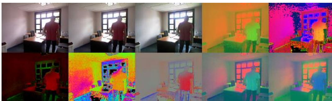
Figure 12. Example of different Colour Models and Invariants. From top-left to bottom-right: RGB (original), Greyworld, RGB-Rank, L^*a^*b^* , HSL, Opposite Colourspace, l1l2l3 , c1c2c3 , YIQ, YCbCr. (Image source: [39]).
