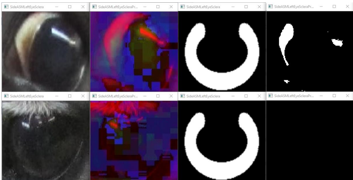
Figure 27. Sclera (eye white) detection by converting the eye feature into the HSV colour space, filtering out irrelevant areas with a shape mask and placing specific thresholds on each channel, leaving a selection of recognized eye white. Both an image with high and low (no) percentage of eye white are shown.
