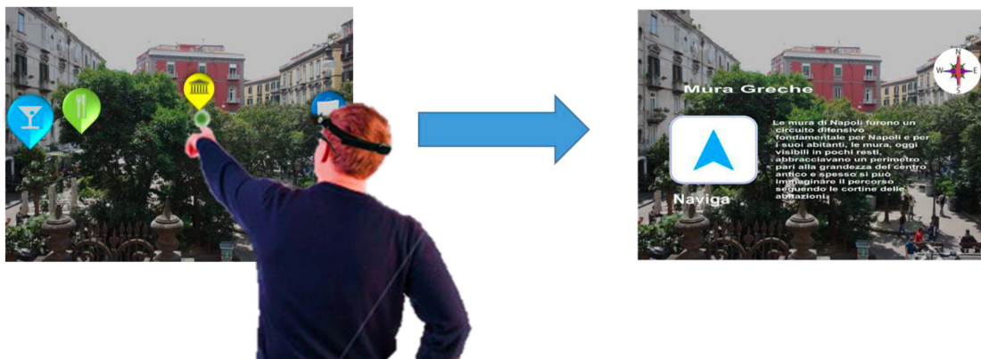
Figure 7: An infographic on the explorative AR system for Napoli. The user selects a POI and can start navigating. Source: Image taken from ICAR citing the paper from Caggianese [16].
