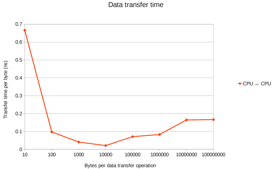
Figure 6.6: A more informative view on CPU to CPU transfers. Again these values are for an NVIDIA Tesla C2050 and an Intel i5.
