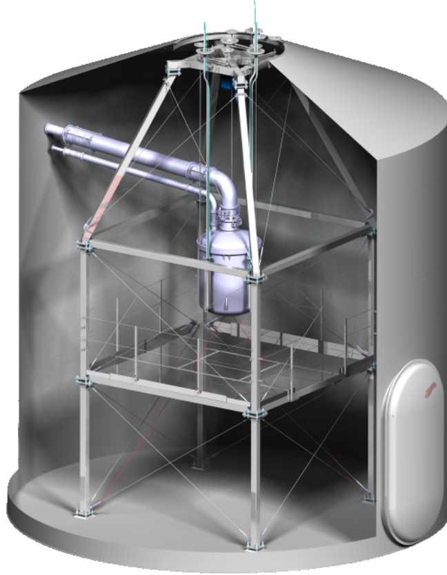
Figure 3.5: A drawing of the water tank of XENON1T containing the support structure holding the cryostat with the TPC. The water tank is over three storeys high.
