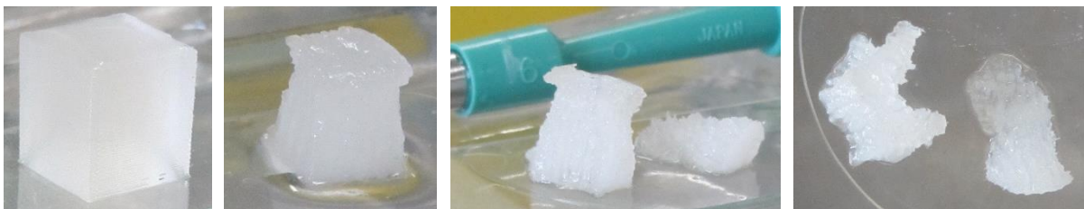
Figure 15: Punching of gelMA construct.
