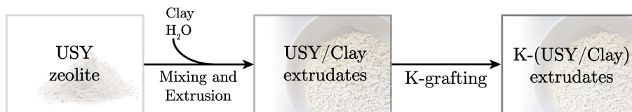
Scheme 1.8: Two-step upscaling procedure proposed for the preparation of technical K-grafted USY/Clay extrudates used in the upgrading of pyrolysis oil.
