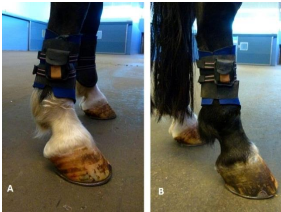
Figure 2. IMU sensors attached to the limbs. A. Fore limbs. B. Hind limb.
