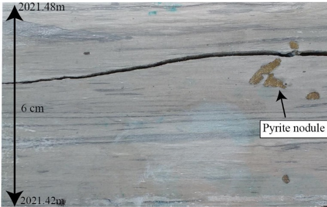
Figure 31. Pyrite nodule inside a laminated grey interval. Left axis is depth in MD
