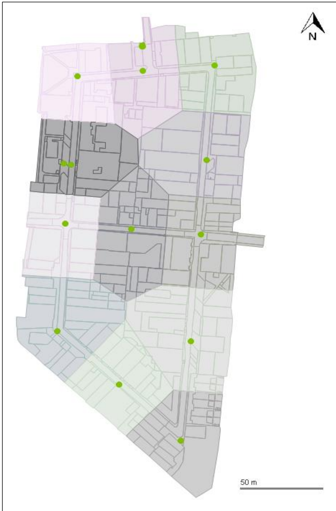
Figure A-5 The division of the island into subcatchments for every manhole (InfoWorks model).
