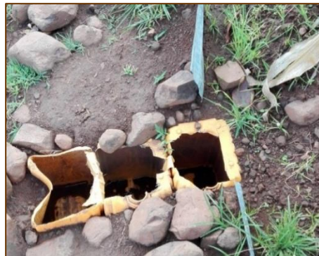
Figure 2-3. Runoff collection jerrycans, downslope of the control plots.
