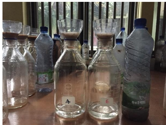
Figure. 3-7. Filtering of sediment of 1L bottles. Samples were taken from the jerrycans below the control plots.
