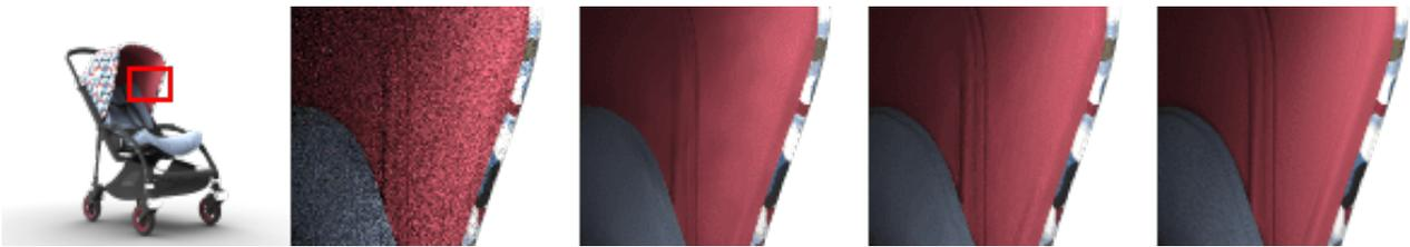
FIGURE 6.2: From left to right: 800ms noisy input, 800ms denoised (spotty shadows), 9600ms denoised (acceptable quality), reference.
