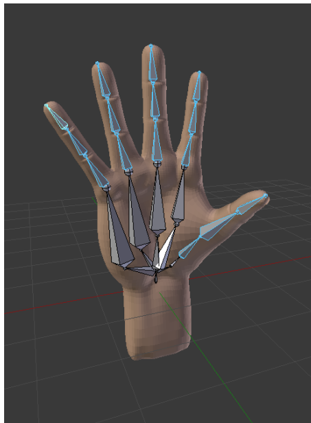
Figure 2.4: A rigged hand. The root of the skeleton is the wrist. From the root originate five chains of bones depicting the digits. The bones that we animate (the phalanges and the thumb metacarpal) are outlined in blue. The black outlined bones (several wrist and metacarpal bones) do not move during the animation; the joints between two static bones are considered rigid.
