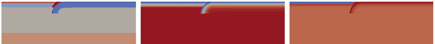
Figure 34: Begin conditions section 3. Left: material field, middle: temperature field, right: density field. Legend same as before.
