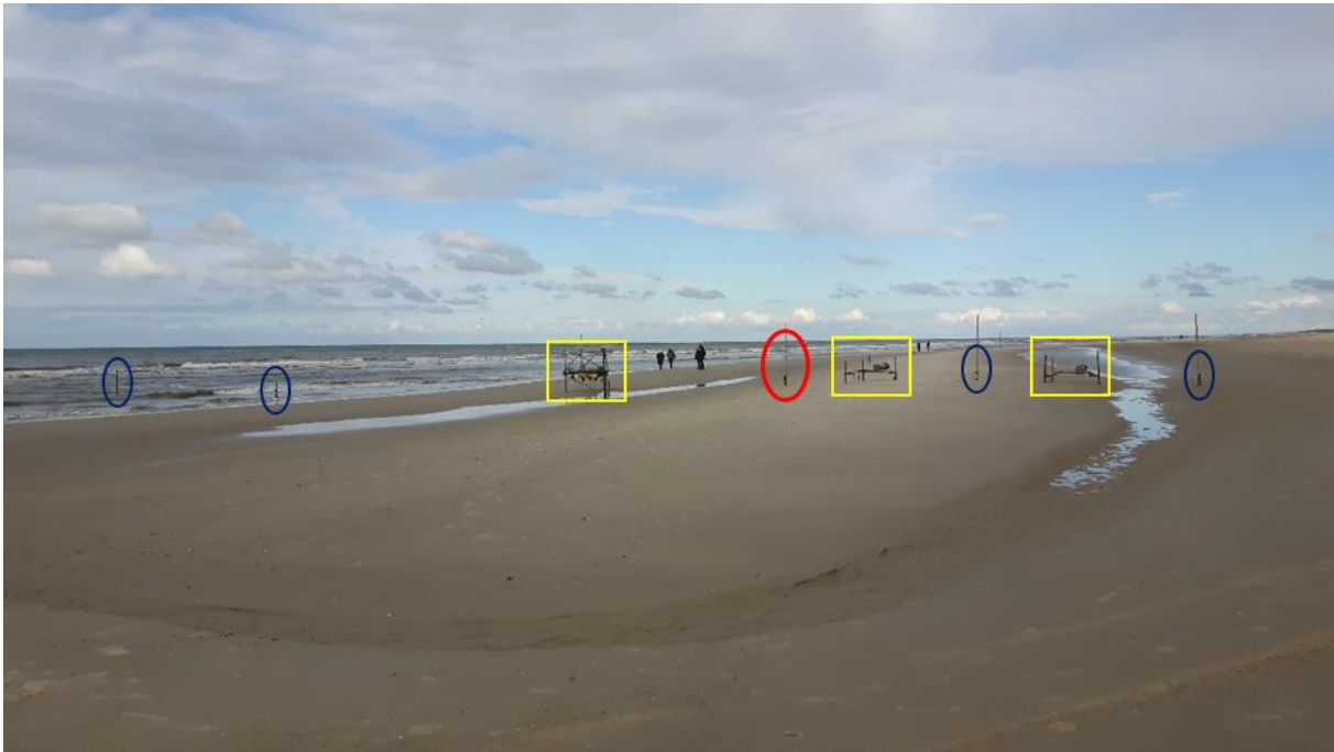
Figure 21: A side picture of the cross-shore array faced towards the north. Indicated are the instruments, with OSSI 3 located within the red oval. Instrument order from left to right: OSSI - OSSI - large-frame - OSSI 3 - mini-frame - OSSI - mini-frame - OSSI.
