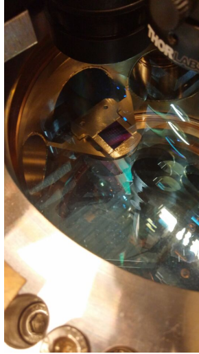
Figure 3.10: The sample containing nanophotonic waveguides placed inside the vacuum chamber.
