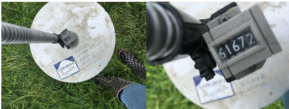
Figure 2. The Jenquip Rising Plate Meter (left) and it's reading plane (right).
