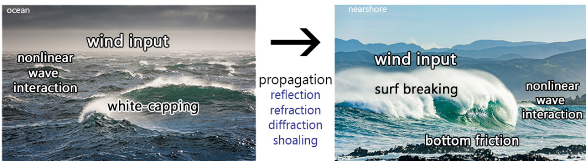
Figure 7: Illustration of physical processes during wave generation and propagation. In the deep ocean, the main sink is white-capping (spontaneous breaking wave), while both of bottom friction and surf breaking dominate the dissipation of energy in the shallow area.
