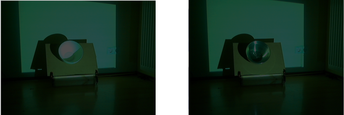
Figure 5.21: The painted and unpainted bowl in the same orientation side by side. Even with the projector not projecting any intentional light, the unpainted bowl already shows a lot of specular light.
