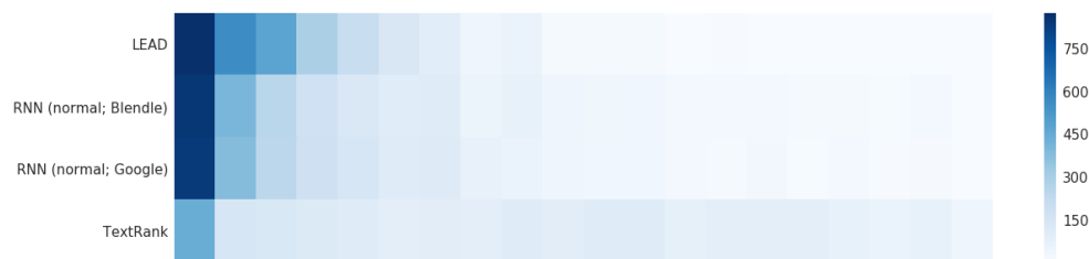
Figure 16: Normalized positional distribution of selected sentences per article for the normally trained RNN models, with the LEAD baseline and TextRank for reference. The number indicates the absolute number of sentences falling in that bin.
