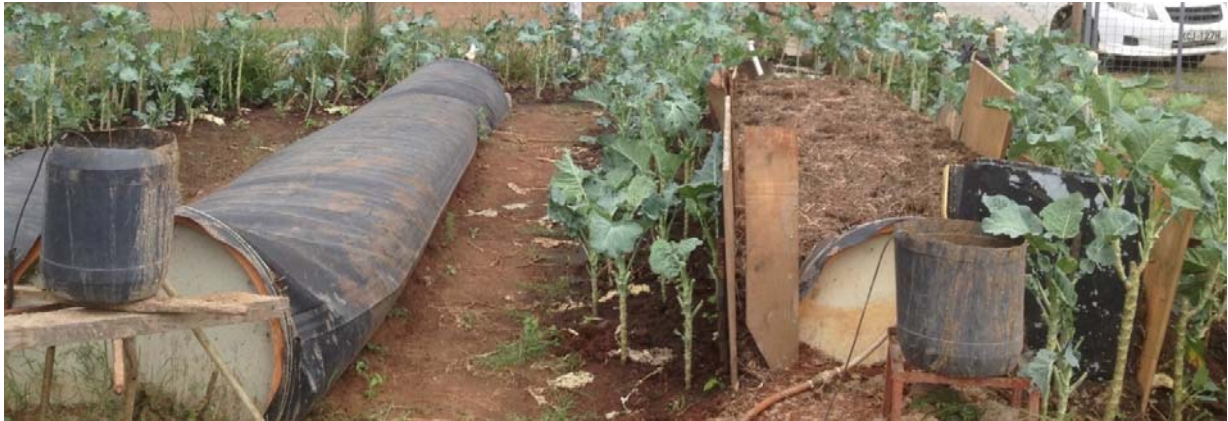
Figure A 6: picture showing the experiment done at the Rehau test site. Of the two identical 3.2 m 3 one is covered with soil (right) to simulate the isolation potential of soil. The other digester is not covered (left). Picture from own archive.
