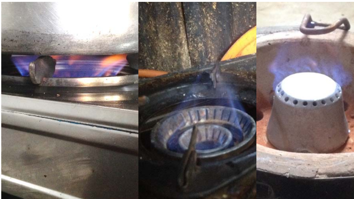
Figure 21: visual observation of the pressure of respectively a brick-dome digester (biodigester 6) a Simgas digester (biodigester 8) and a Rehau digester (biodigester 12), through the observation of flame strength. Pictures from personal archive.
