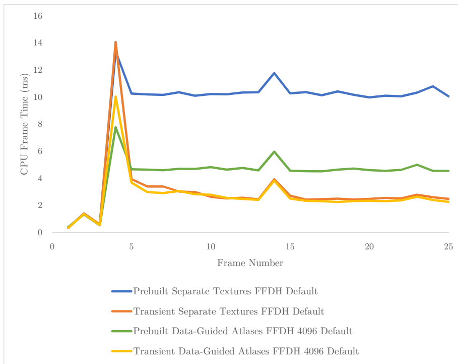
Figure 5.1: The average number of CPU frame time in milliseconds spent on the render thread over 25 frames for a selection of configurations ran with simulation 2.
