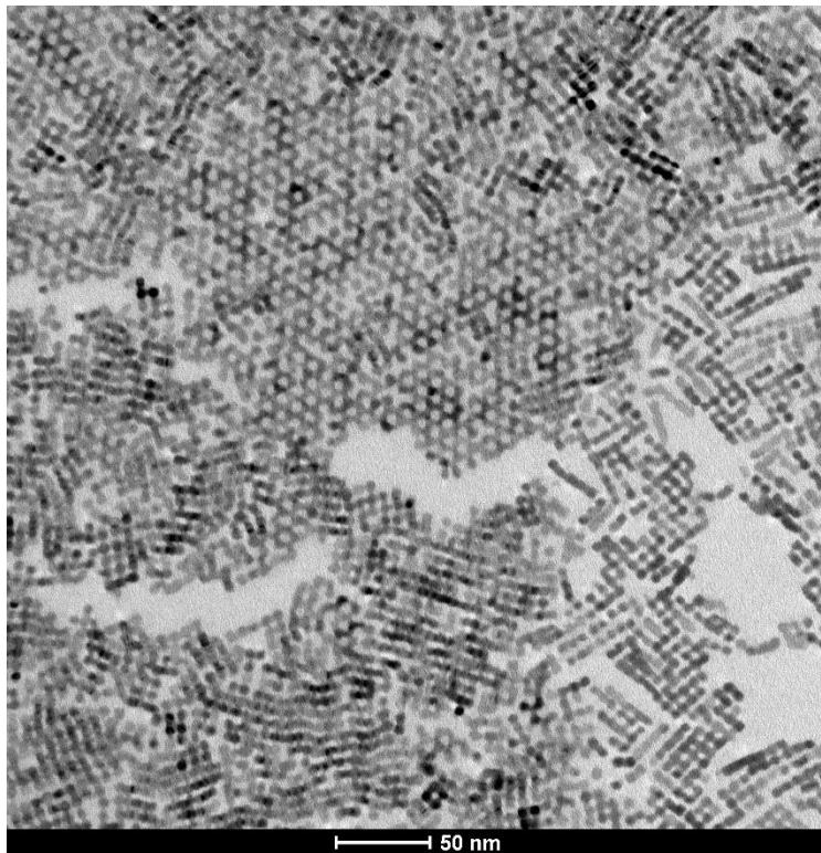
Figure 5-18: The amount of honeycombs seems to increase when less oleic acid is used
