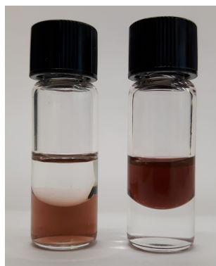
Figure 6.2: Photograph of the particles before (left) and after (right) OTMS-functionalisation. The top and bottom phase are toluene and H 2 O respectively. The vials were vortex-mixed and left to phase separate before taking the image. The darker colour after functionalisation is due to a higher particle concentration.
