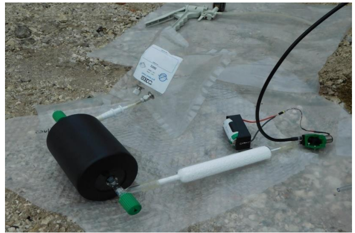
Figure 3: Photograph of gas sampling set-up.
