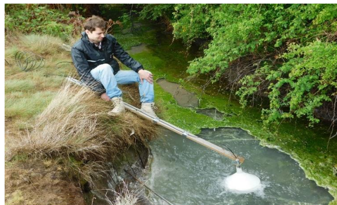
Figure 6: Sampling set-up for wet sources.
