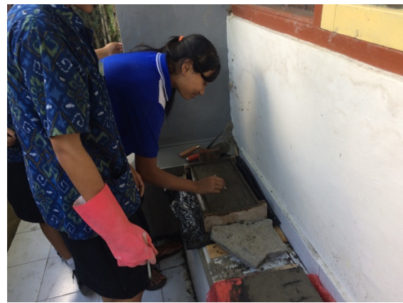
Figure 24: Students of the tourism high school making cement bricks with plastic inside them
