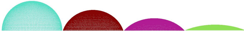
FIGURE 6.7: Drop models created with a spherical cap at 0.5, 0.6, 0.7 and 0.8 of a unit sphere.
