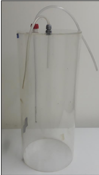
FIGURE 12: THE STATIC CHAMBER USED FOR THE EXPERIMENT
