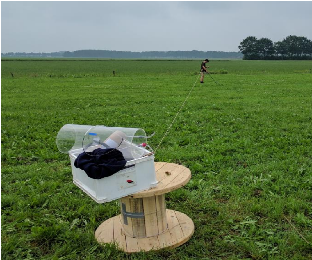
FIGURE 11: PHOTOGRAPHY OF THE PRACTICER MEASURING METHANE CONCENTRATION IN A 16 METERS RADIUS CIRCLE, THE WOODEN SPOOL BEING LOCATED AT THE EXACT X-Y COORDINATES OF THE WELL (PHOTO TAKEN IN JULY 2017)
