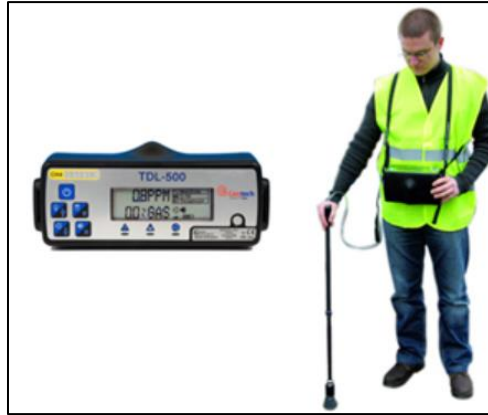
FIGURE 10: METHANE DETECTOR USED DURING THE EXPERIMENT (STIEBER, 2017)
