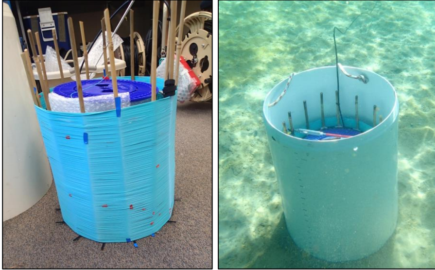
Figure 4.6: Vertical FO-DTS device created from unarmored fibre optic cable and bamboo in lab (left) and installed inside a PVC cylinder during deployment in Whakaipo Bay
