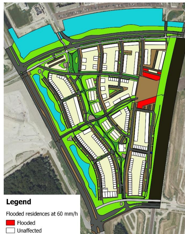
Figure 4-2. Flooded residences at 60 mm/h.
