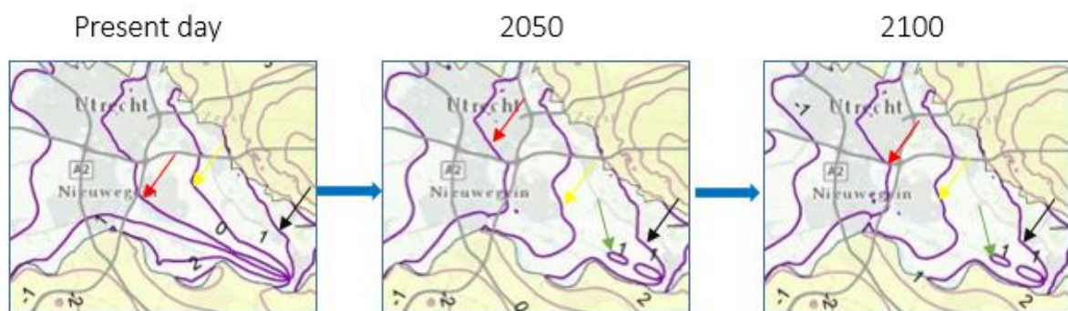
Fig. 17 Enlargement of the Prinses Irene sluices in the Amsterdam-Rhine canal, based on data presented in Fig.16, over the contour lines in the first aquifer. To get a better visualization of how the contour lines shifts from present day to 2050 and 2100, they have been assigned a colour in figure 17; red represent the contour line for 0 m NAP, Yellow 1 m+ NAP, Black 2 m+ NAP and Green >1 m+ NAP.
