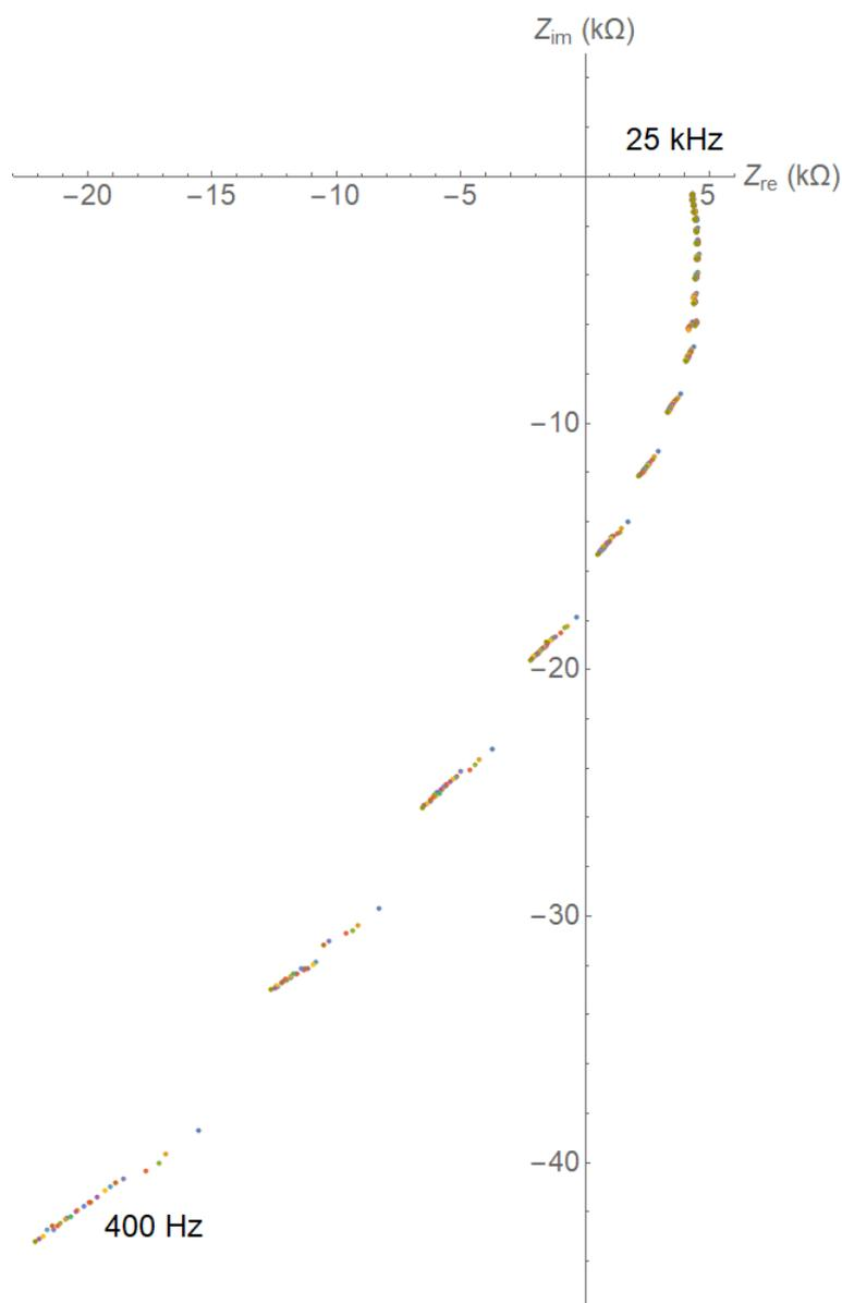
Figure 4.10: Impedance in the complex plane, for 25 EIS measurements in the sensor compartment, while the carbon membrane is electrified. Each colour represents a measurement, for each measurement all frequencies are shown simultaneously.
