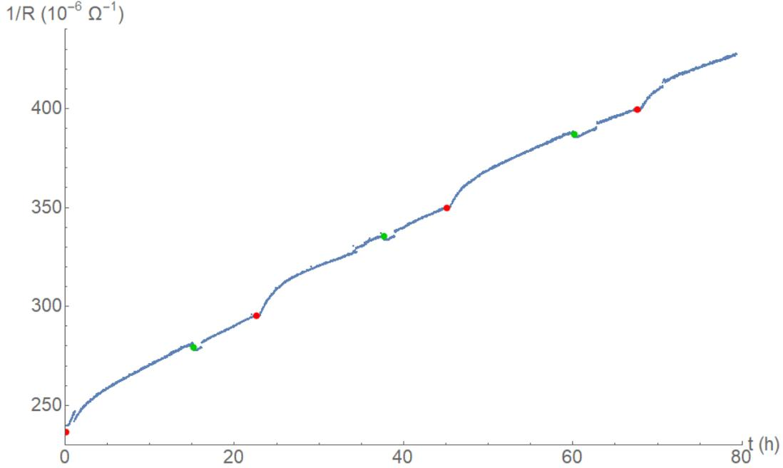
Figure 4.6: Conductance ( $1/R$ ) of solution in the sensor compartment, over time, while the carbon membrane is electrified. Blue points are the values obtained from fitting the EIS data. The green dots indicate when the potential of the carbon membrane is increased, the red dots indicate when extra salt is added to the bulk compartment.
