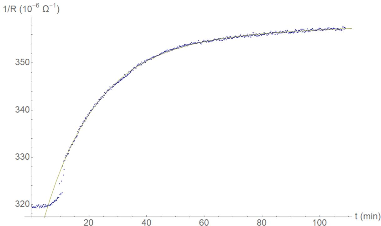
Figure 4.4: Conductance ( $1/R$ ) of solution in the sensor compartment, over time. Blue points are the values obtained from fitting the EIS data. The yellow line is fitted as exponential decay, with linear background.
