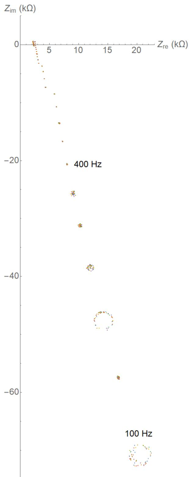
Figure 4.8: Impedance in the complex plane, for 50 EIS measurements on a 0.1 M NaCl solution in the sensor compartment. Each colour represents a measurement, for each measurement all frequencies are shown simultaneously.
