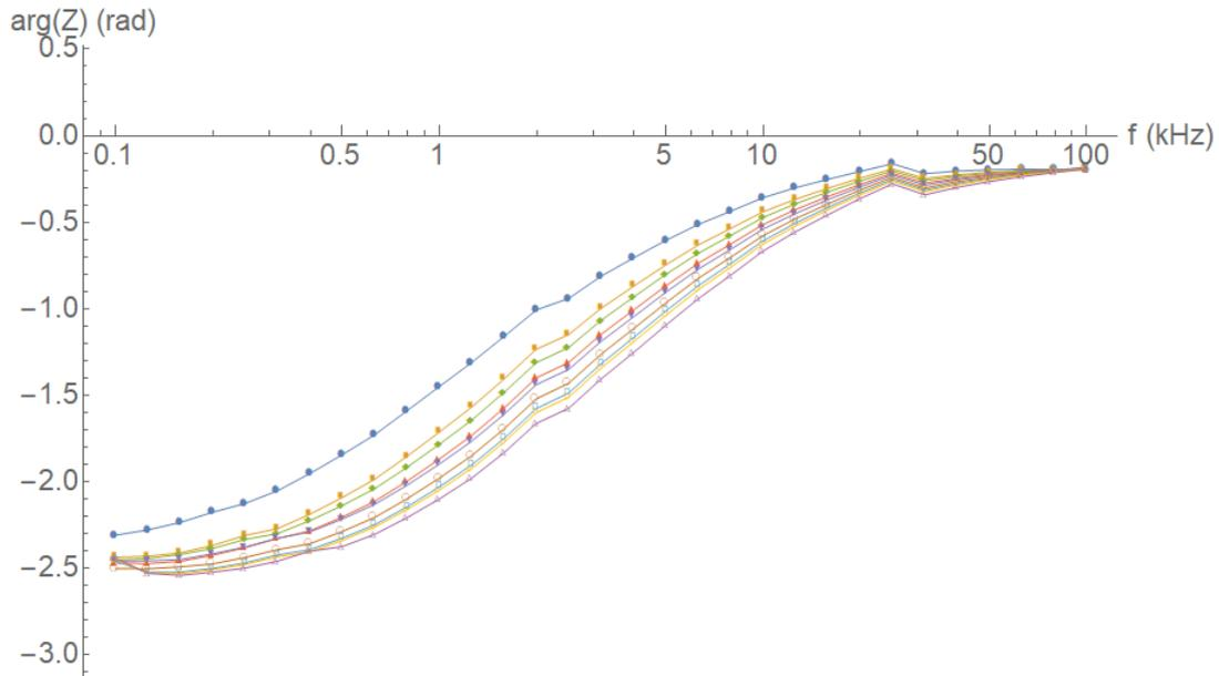
Figure 4.5: Impedance phase vs frequency, for 9 EIS measurements in the sensor compartment while the carbon membrane is electrified. Each colour represents a measurement. Noticeable are discontinuities around 2 kHz and 30 kHz.
