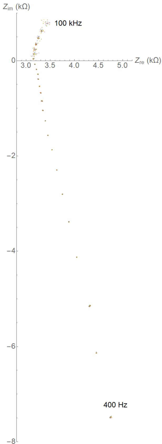
Figure 4.9: Impedance in the complex plane, for 25 EIS measurements in the sensor compartment, before extra salt is added. Each colour represents a measurement, for each measurement all frequencies are shown simultaneously.
