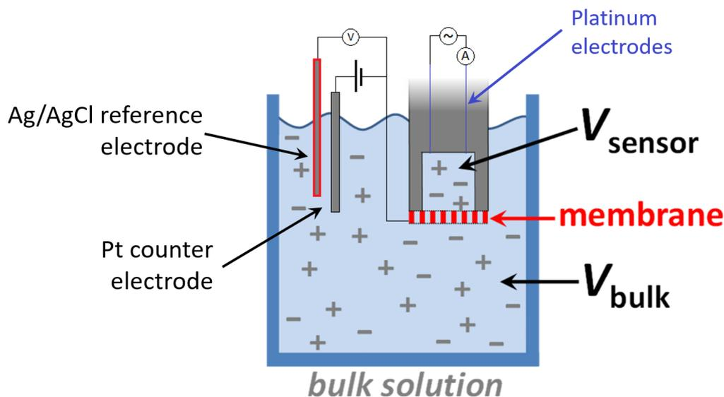
Figure 3.3: Schematic view of charge sensor setup (reproduced from [2]). The Ag/AgCl reference electrode and Pt counter electrode are used to charge the porous carbon membrane. The platinum electrodes in the sensor compartment are used to determine the salt concentration.
