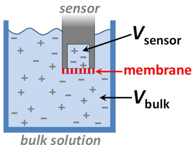
Figure 3.1: Schematic view of charge sensor setup (reproduced from [2]). The setup is filled with an aqueous NaCl solution.
