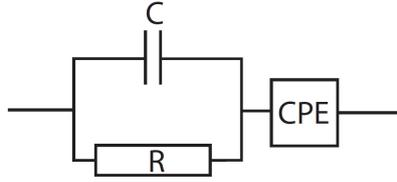
Figure 3.4: Circuit used to model the NaCl solution between the platinum tips.
