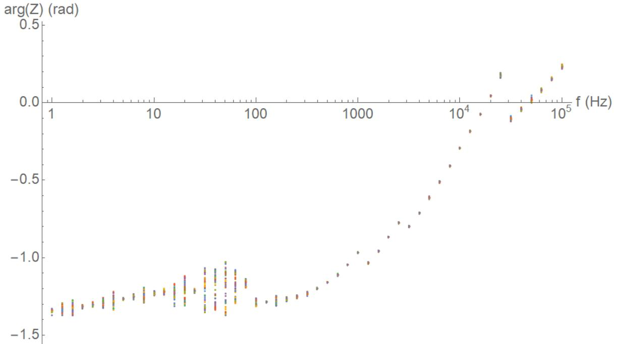
Figure 4.3: Impedance phase vs frequency, for 50 EIS measurements on a 0.1 M NaCl solution in the sensor compartment. Each colour represents a measurement. Noticeable is the low precision below 100 Hz, and a few discontinuities at higher frequencies.
