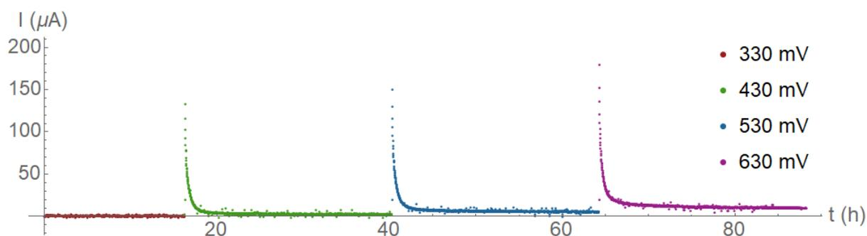
Figure 4.1: Current while charging the porous carbon membrane in aqueous NaCl solution at various potentials vs Ag/AgCl. The NaCl concentration ranged from 1 mM to at least 40 mM.
