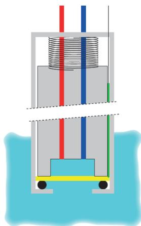
Figure 3.2: Schematic view of sensor probe (reproduced from [8]). The yellow membrane represents the porous carbon membrane, the green line a pencil lead used to make the electrical contact. With conducting glue, the lead is glued to a copper wire (in black).
