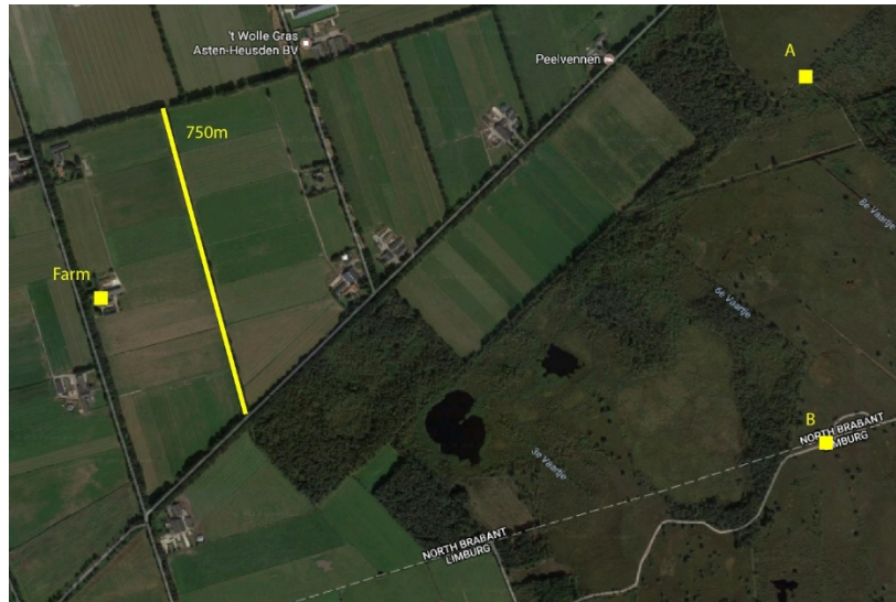
Figure 1: Satellite image of the survey area, with the 750 receiver line colored yellow. The equipment was controlled from the farm slightly west of the line. Points A and B represent the locations of two borehole surveys. From Google Maps (2017).
