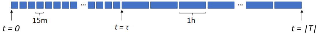
Figure 10: Graphical representation of the change in time resolution. The time steps up to t = \tau will be 15 minutes long, while all time steps after that will be considered in groups of four, in other words: the time resolution changes to 1 hour per time step.
