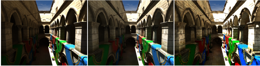
FIGURE 4.4: A pathtraced render of Sponza using one point light as a sun (left), compared to our approach using indirect illumination maps (middle) and our composite light map approach (right).
