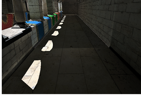
FIGURE 3.7: Two grid cells near the camera have switched over the next level of detail. A border is visible between the grid cells that are at the lower LOD level and those that are at the higher level. The image has been brightened for the purpose of comparison.
