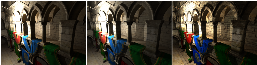
FIGURE 4.5: A pathtraced render of Sponza using two point lights (left), compared to our approach using indirect illumination maps (middle) and our composite light map approach (right).
