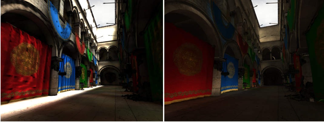
FIGURE 3.2: The radiance map visualized directly on the Sponza scene (left), containing global illumination. A visualization of the final gather map, containing indirect illumination only (right).
