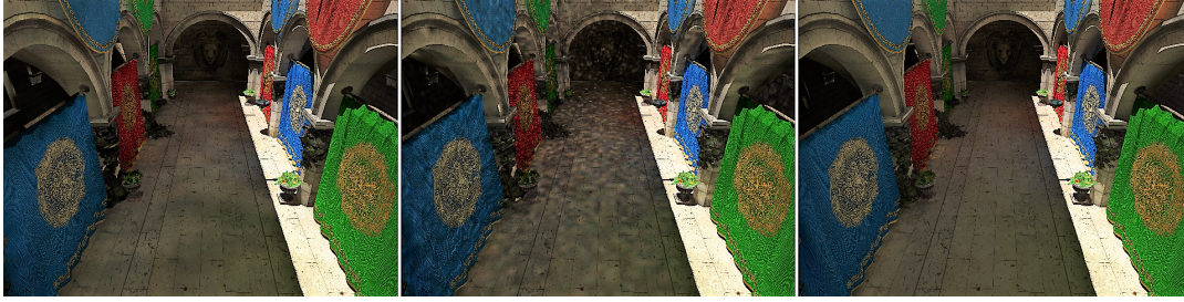
FIGURE 3.4: A visualization of the view-based updates. The left image shows initial lighting, computed using eight FG rays. The middle image shows lighting being updated by casting additional FG rays. The right image shows the converged result, as enough FG rays have been cast for detailed lighting. The image has been brightened for the purpose of comparison.
