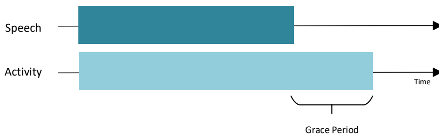
Figure 6.2: An actor remains classified as active for a brief period of time proceeding its latest speech. This to account for natural pauses between consecutive utterances.
