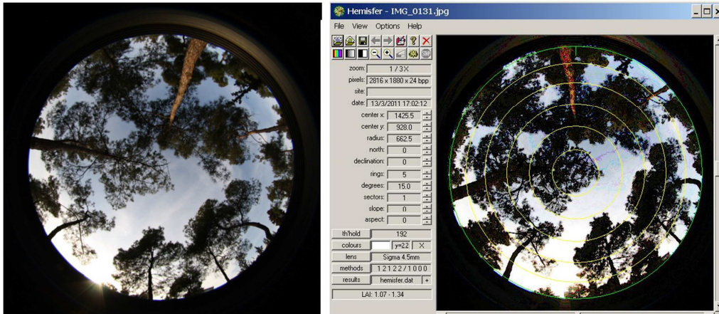
Figure 14: Hemispherical photograph in RGB and processing with specialized software.
