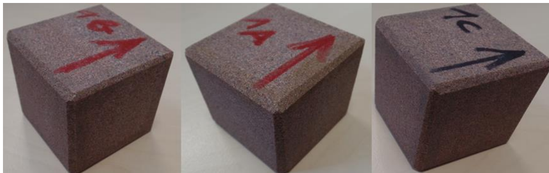
Figure 2 Three cubes of the Bebertal sandstone before applying deviatoric and hydrostatic stress (left) KB-1b, (middle) KB-1a, and (right) KB-1c.
