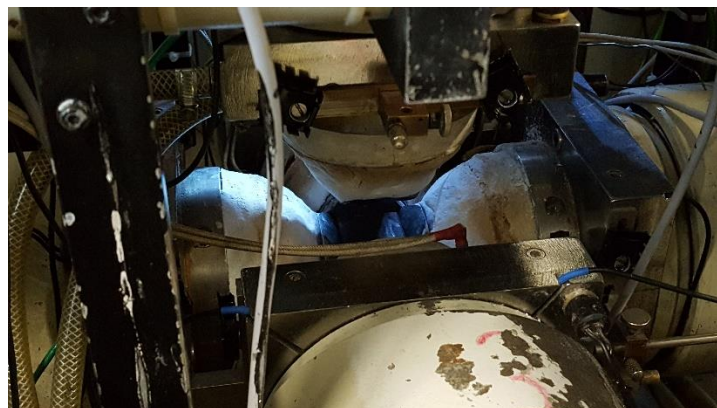
Figure 4 Six pistons from the sample is in process of being pressurized by six pyramidal pistons in three orthogonal direction.
